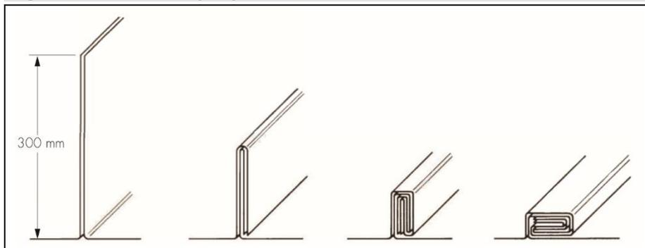
13.3 Alternatively, when it is not possible to keep the membrane dry, a double-welted fold should be formed using at least 300 mm of the membrane (see Figure 2). The dpm must be continuous with the dpc in the surrounding walls. Where necessary, the membrane should be used as a vertical dpc to link the two. It is essential that the fold is held in position prior to placing the concrete, eg by weighting with bricks.
