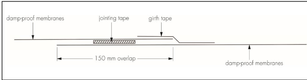
13.2 The dpm must be continuous and linked in with the damp-proof course (dpc) in the surrounding walls. Where necessary, the products should be used as a vertical dpc to link the two. The dpm and dpc joint must be overlapped by a minimum of 150 mm and sealed with an appropriate jointing tape and girth tape. Where there is doubt about the compatibility of materials, the advice of the Certificate holder should be sought.
